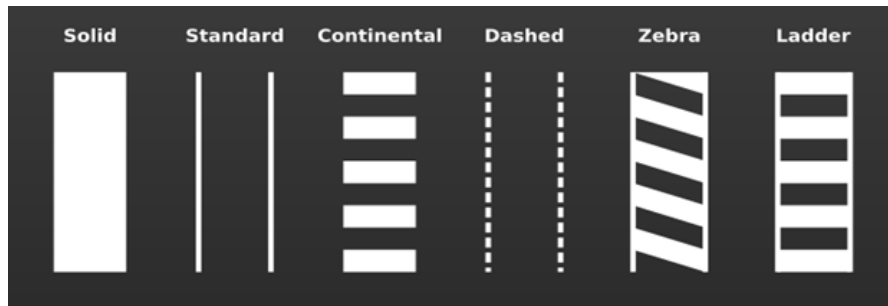
Standard Crosswalk Marking Patterns
